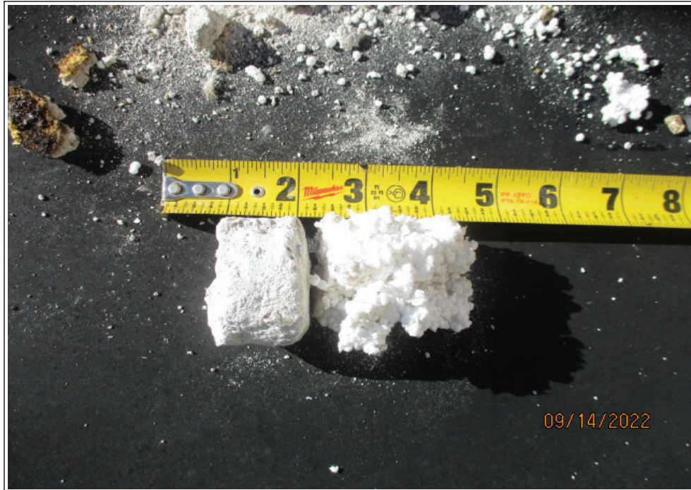
1. AREA "ER": VIEW OF ROOF CORE - EPDM SINGLE PLY MEMBRANE, LWIC, EPS BOARD, METAL FORM DECK
