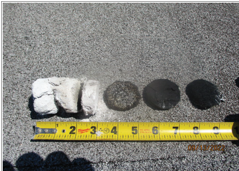
4. AREA "N4": VIEW OF ROOF CORE - MODIFIED BITUMEN MEMBRANE, BASE SHEET, LWIC, EPS BOARD, METAL FORM DECK
