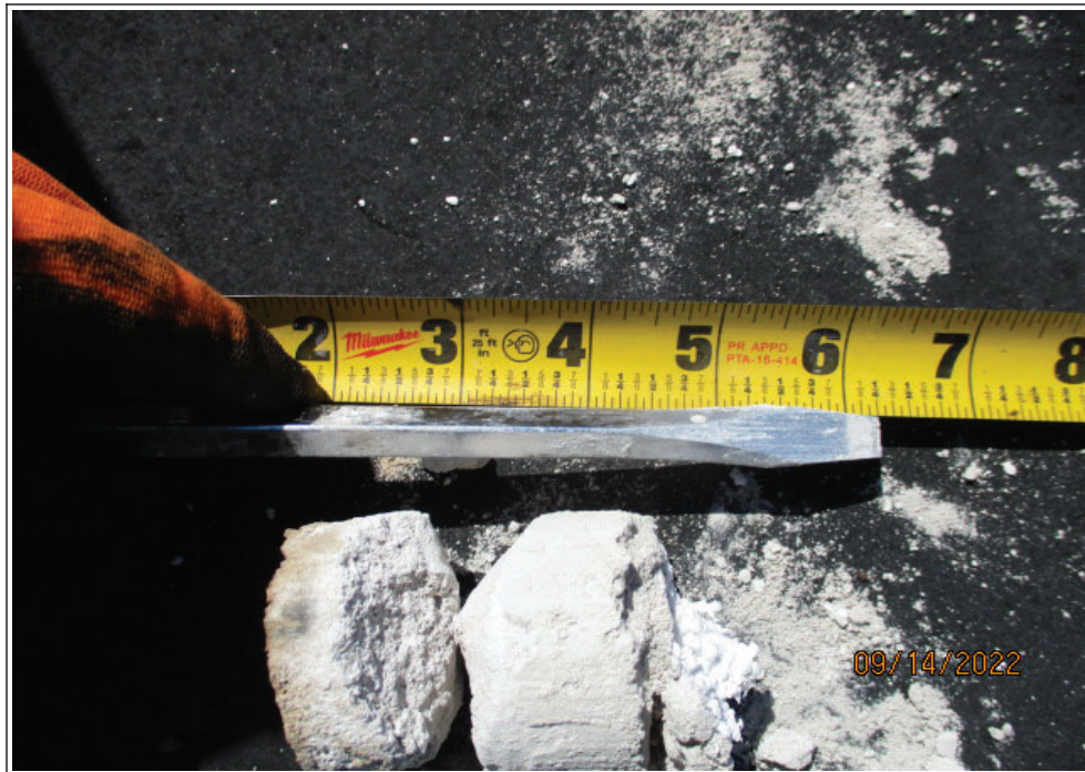
5. AREA "S3": VIEW OF ROOF CORE - EPDM SINGLE PLY MEMBRANE, LWIC, EPS BOARD, METAL FORM DECK
