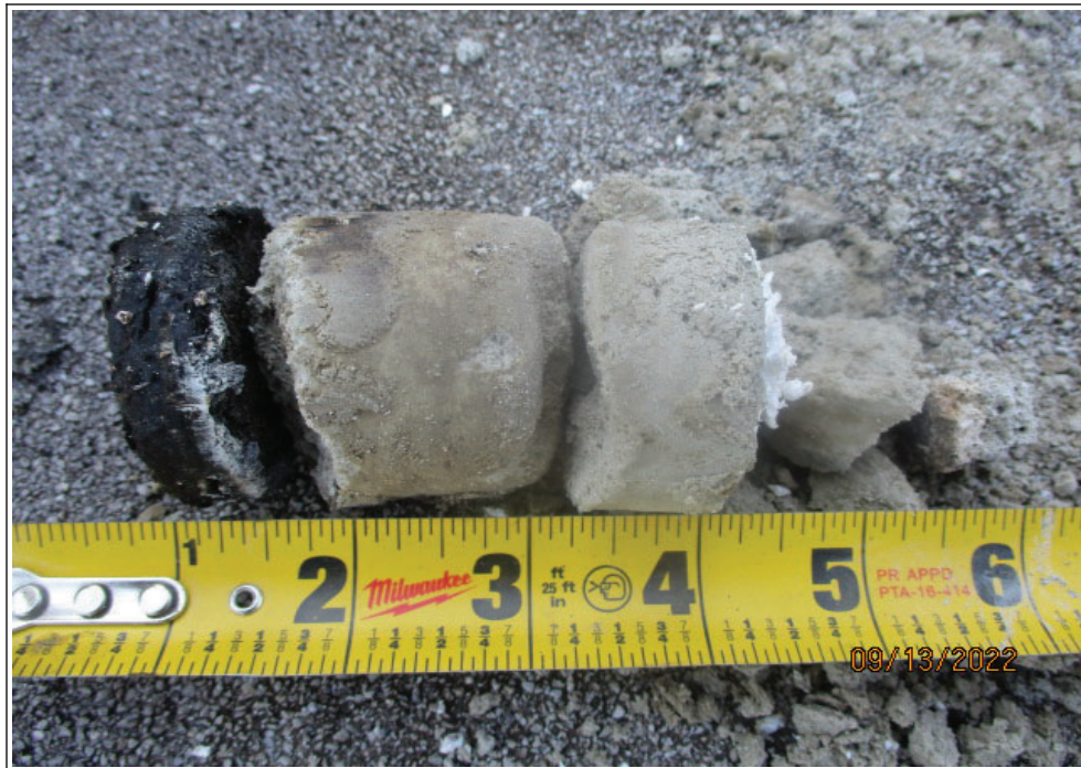
3. AREA "N3": VIEW OF ROOF CORE - MODIFIED BITUMEN MEMBRANE, BASE SHEET, LWIC, EPS BOARD, METAL FORM DECK
