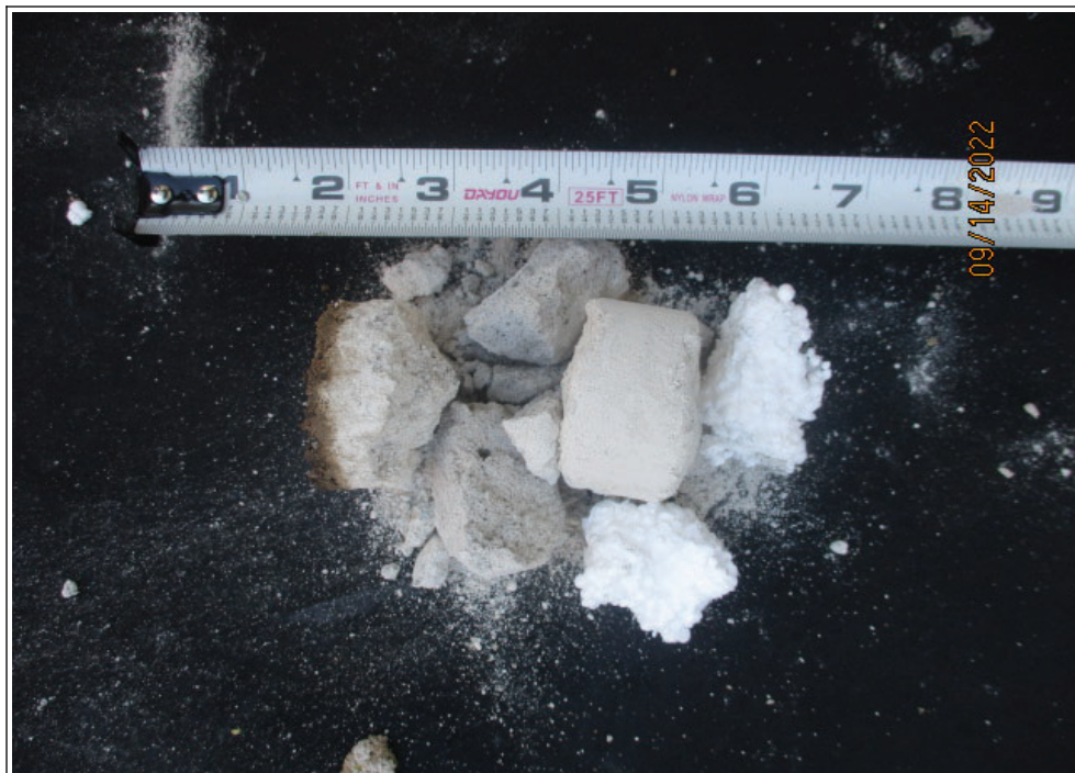
6. AREA "ER": VIEW OF ROOF CORE - EPDM SINGLE PLY MEMBRANE, LWIC, EPS BOARD, METAL FORM DECK
