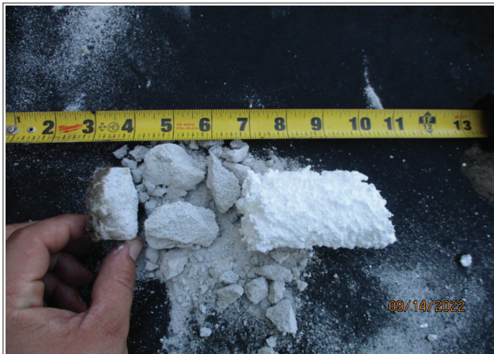
6. AREA "S4": VIEW OF ROOF CORE - EPDM SINGLE PLY MEMBRANE, LWIC, EPS BOARD, METAL FORM DECK
